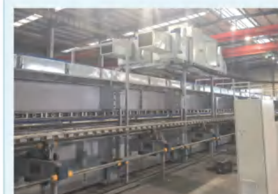
湖南本土企业 聚氨酯连续板材生产线 Hunan Local Enterprise: Polyurethane continuous sandwich panel production line
